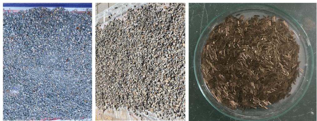
**Figure 1.** In-site photos of raw materials: NAs, natural coarse aggregates (left); RAs, recycled coarse aggregates (middle); BF, basalt fiber (right).
