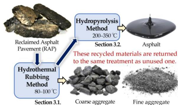
Figure 2. Separate recycling technology.
