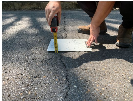
Figure 1. Bridge end bump problem caused by settlement of an embankment fill.
