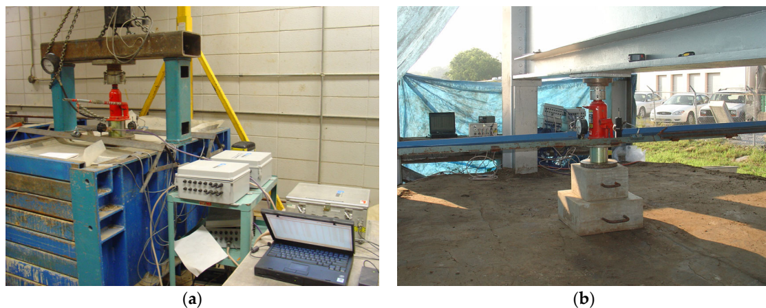
Figure 3. Model footing test setup. (a) Laboratory model test setup; (b) Large-scale field model test setup.
