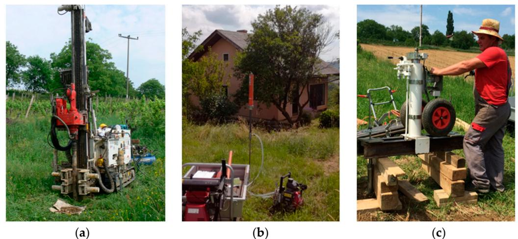
**Figure 6.** Geotechnical in situ investigation equipment: (a) boring machine Comacchio Geo 205; (b) DPL Nordmeyer Geotool PR 30; (c) Hydraulic embossing equipment Hyson LW100.
