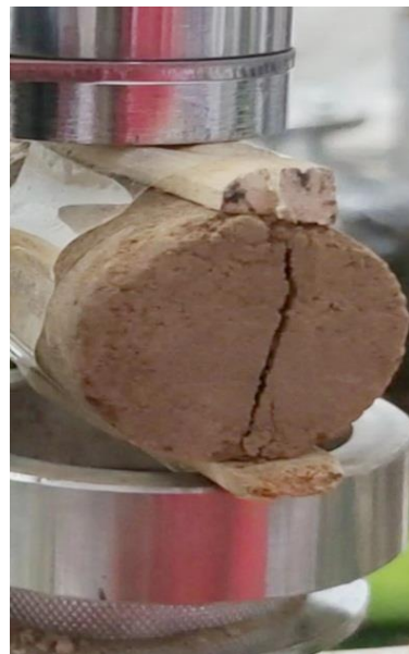
Figure 3. Indirect tensile test.
