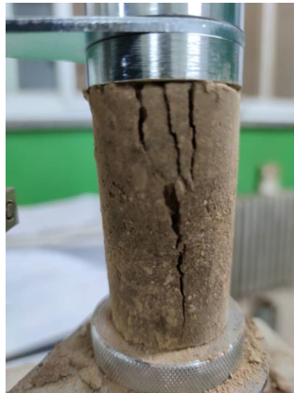
Figure 2. Unconfined compressive test.
