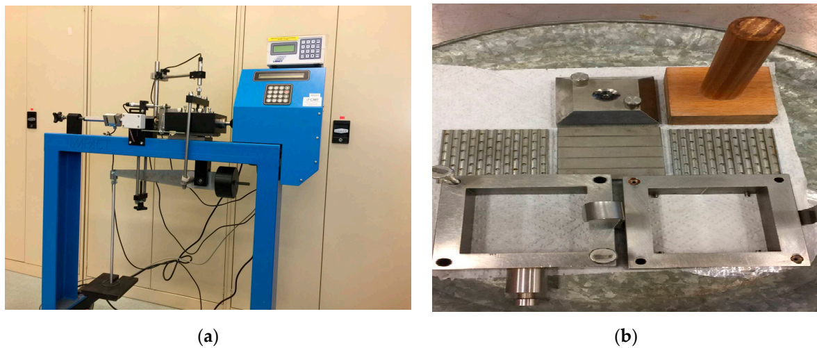
Figure 1. Shear box apparatus: (a) shear box apparatus and data log; (b) 60 mm × 60 mm shear box.
