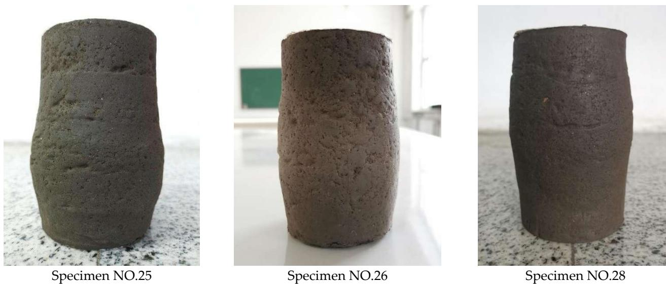
**Figure 16.** Appearances of tested specimens going through 11 FTHs.
