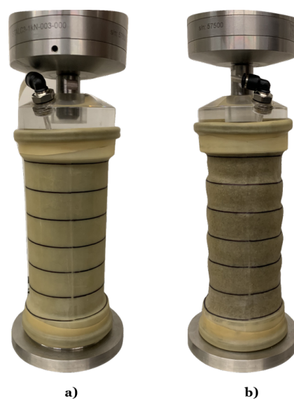
Figure 12. Soil specimens after remoulding: (a) specimen with a ‘zig-zag’ pattern; (b) regular specimen.
