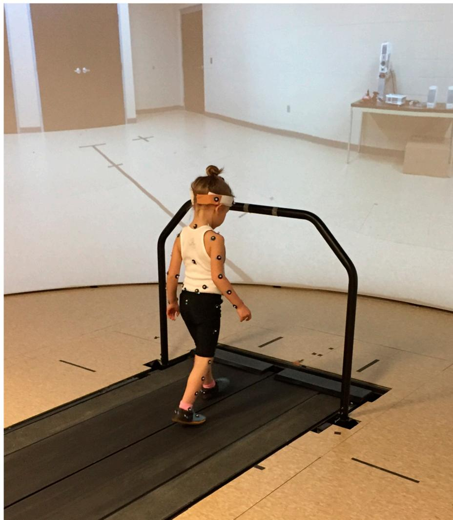
**Figure 1.** Example of child subject walking on the split-belt treadmill. The image depicts a full marker set; however, for this study, only the heel and toe markers on each foot were used to quantify the stride length and stride time for each subject.
