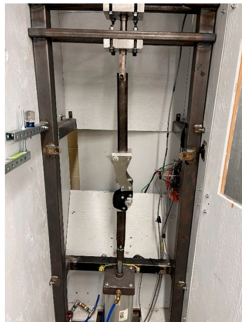
Figure 3. GKnee placed in the pneumatic compression testing rig locked at full extension.
