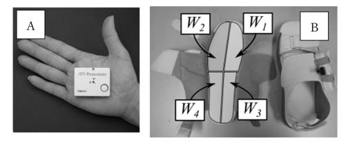
**Figure 2.** Measurement device. (**A**). The Inertial Measurement Unit; (**B**). The foot pressure sensors; W1: forward-right, W2: forward-left, W3: backward-right, W4: backward-left.
