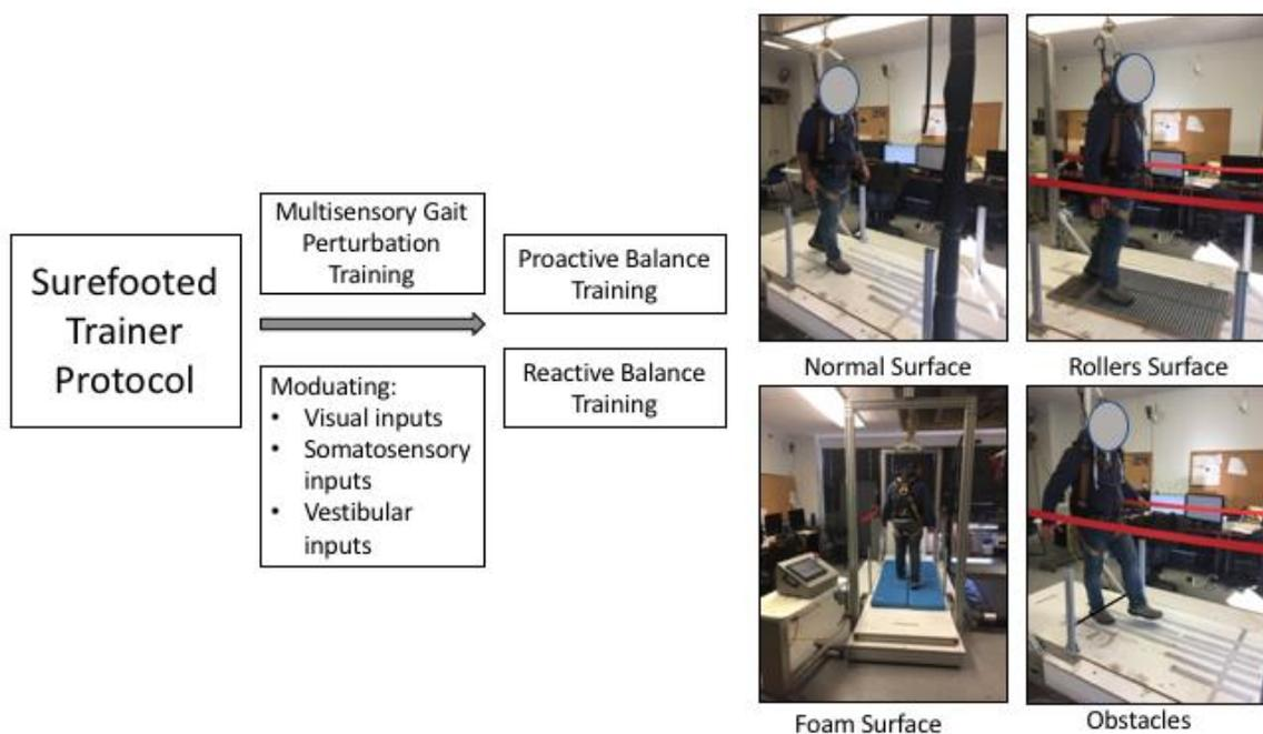
**Figure 1.** Experimental setup and conceptual framework of the computer-controlled movable platform device (Surefooted Trainer). Forward (Slip-perturbation) and backward (Trip-perturbation) platform displacement was provided for each protocol condition.
