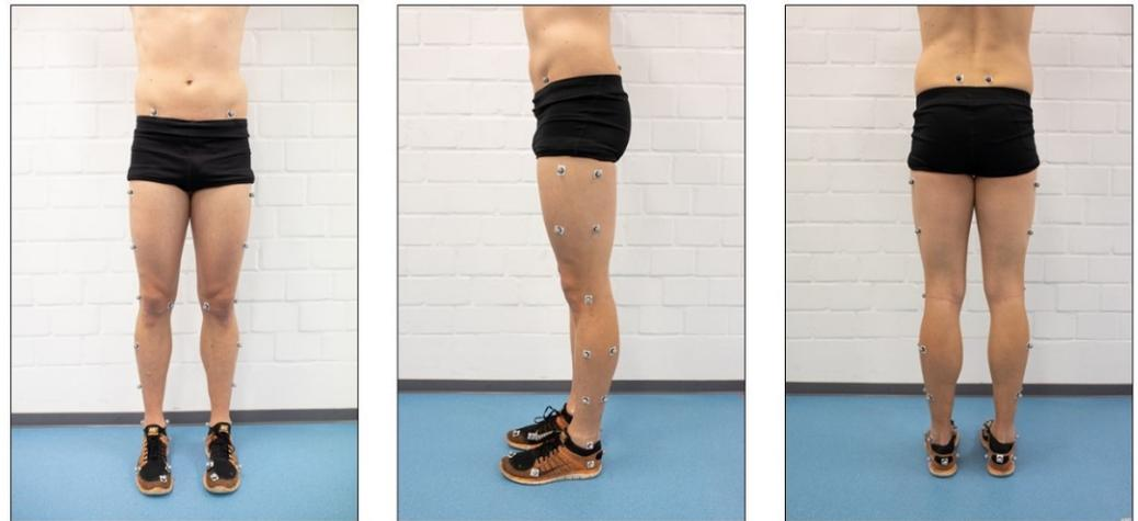
**Figure 4.** Lower-body marker set-up used for 3D motion analysis.
