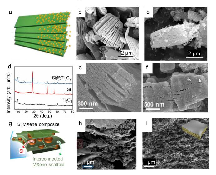
**Figure 3.** Layer-by-layer structured Si/MXene nanocomposites. (a) Schematic illustration of Si/Ti<sub>3</sub>C<sub>2</sub>. SEM images of (b)  $Ti_3C_2$  and (c) Si/Ti<sub>3</sub>C<sub>2</sub>. (d) XRD patterns of Si,  $Ti_3C_2$ , and Si/Ti<sub>3</sub>C<sub>2</sub>. SEM images of (e) MXene/Si and (f) MXene/Si@SiO<sub>x</sub>@C-2. (Reprinted with permission from Ref. [47], Copyright 2018 Elsevier; reprinted with permission from Ref. [48], Copyright 2019 ACS Publishers, respectively).
