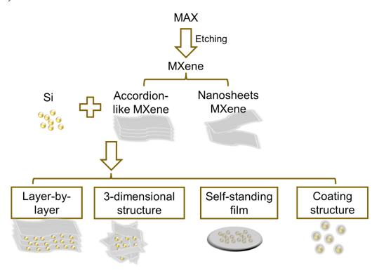
Figure 2. Schematic of the syntheses of Si/MXene composites with different structures.
