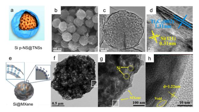
**Figure 6.** Coating structures of Si/MXene composites. (**a**) Schematic illustration, (**b**) SEM, (**c**) TEM, and (**d**) HRTEM images of the Si@MXene composite. (**e**) Schematic illustration and (**f**–**h**) TEM images of Si@MXene capsule. (Reprinted with permission from Ref. [64], Copyright 2020 ACS Publishers. Reprinted with permission from Ref. [65], Copyright 2020 ACS Publishers).
