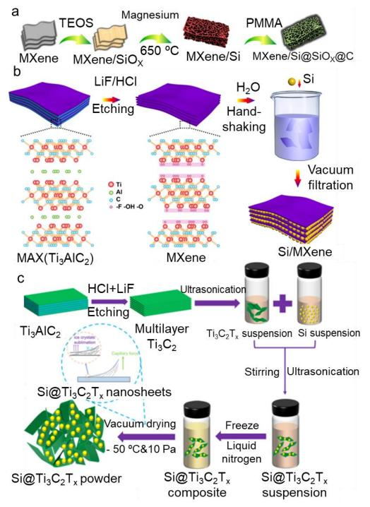
**Figure 8.** Preparation of Si/MXene composites. (a) Schematic preparation procedure for MXene/Si@SiO<sub>x</sub>@C nanohybrids. (Reprinted with permission from Ref. [48], Copyright 2019 ACS Publishers). (b) Schematic preparation routs for Si/MXene composite paper and (c) Si@Ti<sub>3</sub>C<sub>2</sub>T<sub>x</sub> powder. (Reprinted with permission from Ref. [54], Copyright 2019 ACS Publishers; reprinted with permission from Ref. [58], Copyright 2021 Elsevier, respectively).
