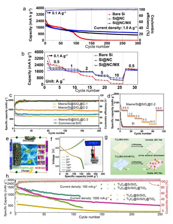
**Figure 12.** (a) Cycling stability and (b) rate capability of the electrodes based on bare Si, Si@NC, and Si@NC/MXene composites. (Reprinted with permission from Ref. [57], Copyright 2021 Elsevier). (c) Cycling performance of MXene/Si@SiO<sub>x</sub>@C-1, MXene/Si@SiO<sub>x</sub>@C-2, MXene/Si@SiO<sub>x</sub>@C-3 and
