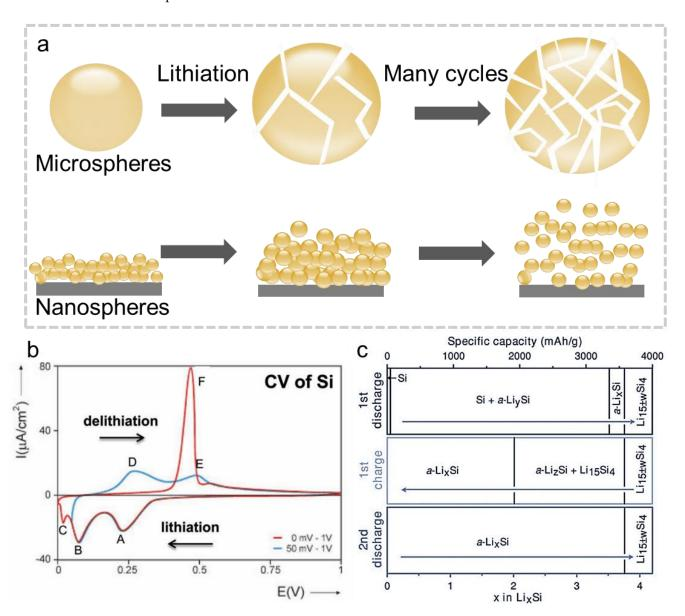
**Figure 1.** (a) Schematic illustration of the failure mechanism during the electrochemical cycling of a silicon negatrode. (b) Typical Cyclic voltammogram (CV) of Si. (c) Phase diagrams at different stages of the charge–discharge cycling of a Li/Si negatrode between 0.005 and 0.9 V at room temperature. (Reprinted with permission from Ref. [6], Copyright 2012 John Wiley and Sons. Reprinted with permission from Ref. [7], Copyright 2007 John Wiley and Sons).
