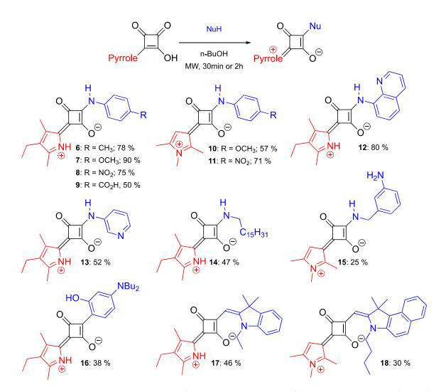
Scheme 4. Synthesis of non-symmetric squaraines from semisquaraines 1a and 4a. Isolated yields are given.
