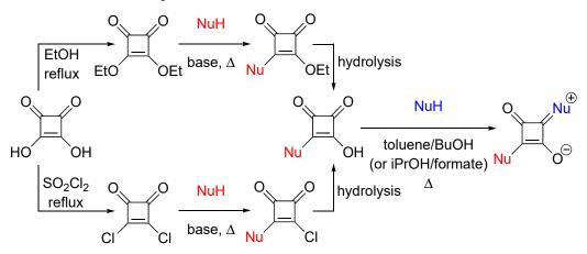
**Scheme 1.** Preparations of non-symmetric squaraines, via diethylsquarate (**top**) or squaryl dichloride (**bottom**), using squaric acid and various nucleophiles (NuH) as the starting materials for each step.
