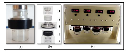
**Figure 2.** In vitro tick feeding system used in this study: (a) feeder device; (b) different parts constituting the feeder: 1. blood-heating lid, 2. blood receptacle, 3. membrane frame, 4. connecter, and 5. tick receptacle; and (c) digital heating power source with four feeding devices.
