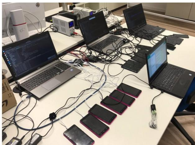
**Figure 2.** Case scenario hardware setup in the first experiment. Each device set (A, B, and C) consists of six devices (1–6) and each device set is controlled by a dedicated laptop (from left to right: Person C, XGody S20 Lite; Person A, Alcatel 1SE; and Person B, Samsung Galaxy A40). One additional laptop (in front) controls the FSM and generates voice messages. The dedicated power supply (in the back) powers the USB hubs and thus charges the devices.
