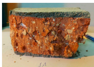
Figure 1. Internal microstructure of the historical brick.
