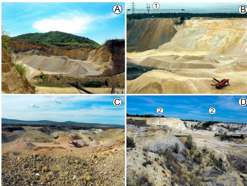
Figure 7. Mine excavated by mechanical mining (A) Márkó mine, (B) Litér mine (C) Kádárta mine (D) Sólly mine. Legend: 1. bauxite fill of the depression of the dolomite, 2. dolomite mound on the strip pit (solid rock is dirt for rubble).
