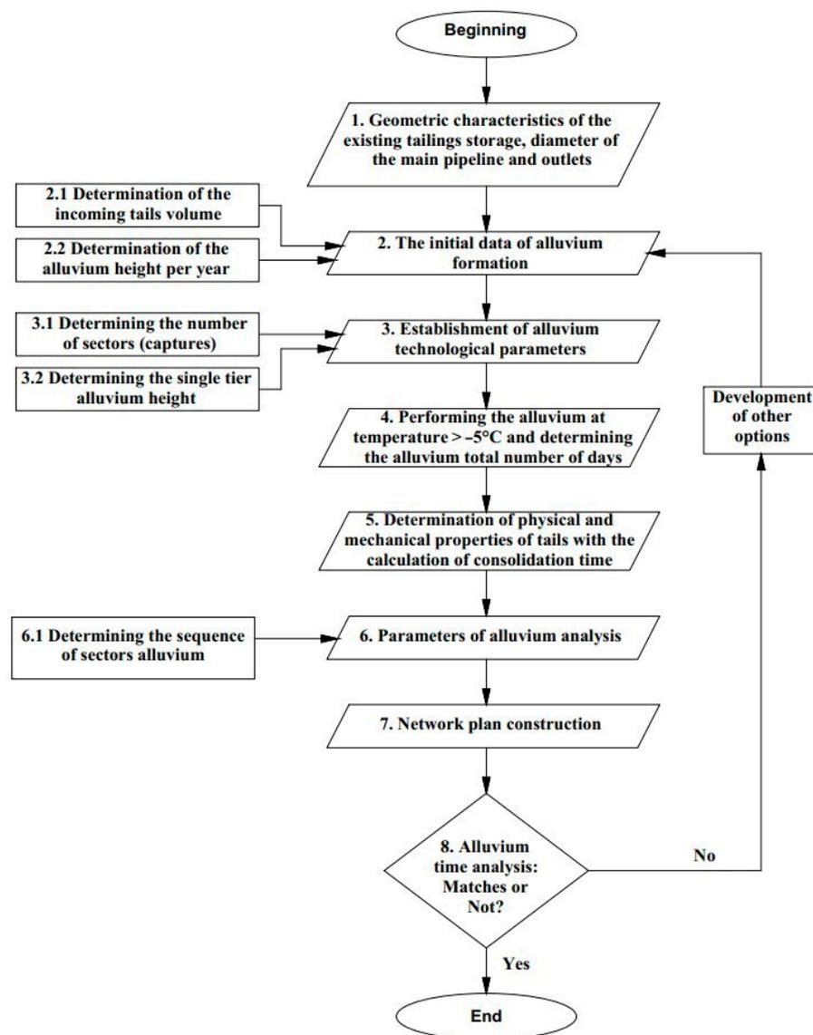
**Figure 7.** The algorithm of tailing dam forming.
