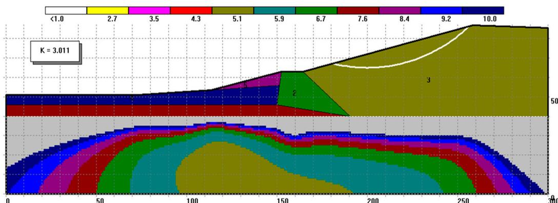
**Figure 23.** The stability coefficient of the enclosing dam after completion of works.
