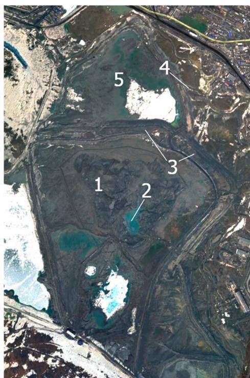
**Figure 2.** Tailing dump №1 (69°20′33.86″ N; 88°7′37.93″ E): 1—tailing dump №1; 2—the pond; 3—local tailing dam; 4—spillway channel; 5—magnetic pyrite depository №2.
