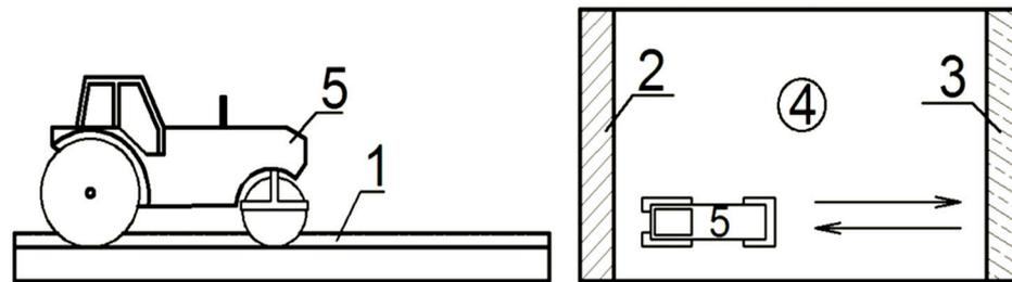
**Figure 18.** The scheme of the compacting process: 1–compacting lay of tails; 2–a retaining prism of a dam; 3–slurry collecting slag prism; 4–a beach zone; 5–roller.
