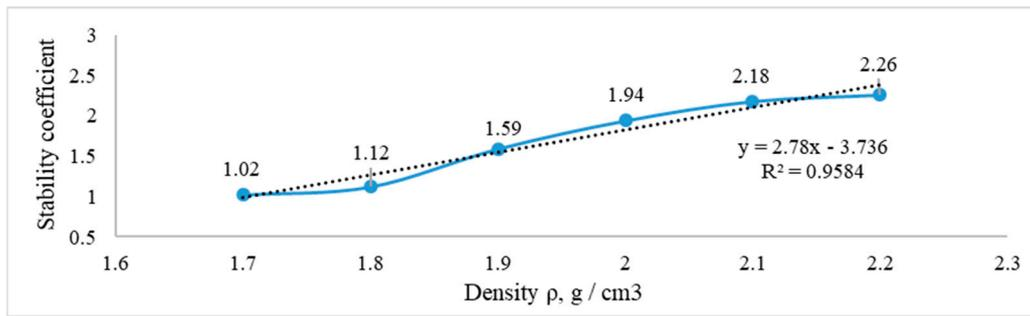
**Figure 15.** The density effect on the dam’s stability factor.
