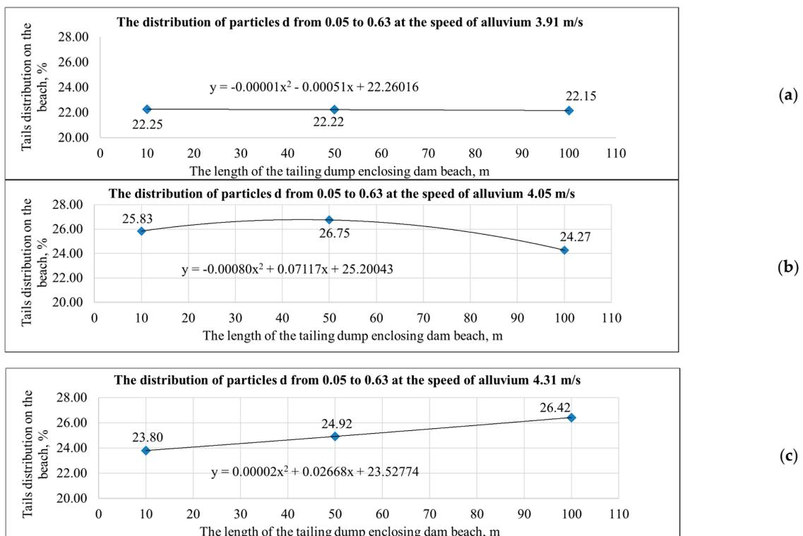
**Figure 11.** The distribution of tails on the beach at speed: (a)  $v = 3.91$  m/s; (b)  $v = 4.05$  m/s; (c)  $v = 4.31$  m/s.
