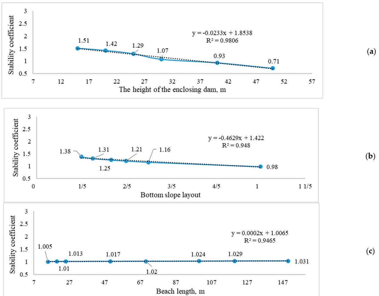
Figure 13. The  $k_{st}$  value depending on the geometrical parameters: (a) the influence of the height of the dam; (b) the bottom slope layout; (c) beach length effect.
