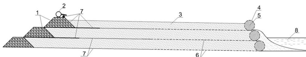
**Figure 10.** The scheme of the dam inwash: 1—enclosing dam in the form of slag prisms; 2—slurry pipeline; 3—tailings beach; 4—separating earth dam in a bay; 5—tails; 6—geotextile filtering material; 7—geotextile non-filtering material; 8—pond.
