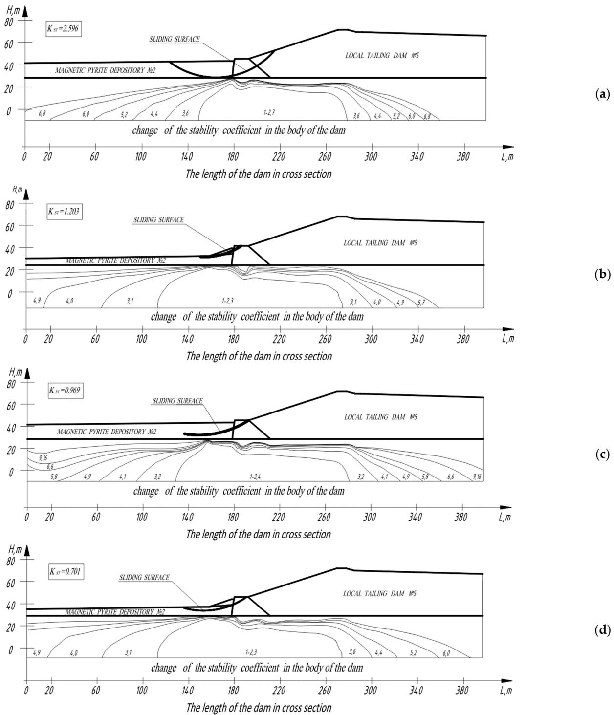
**Figure 22.** Results of stability coefficient calculations: (a) in winter time prior to the beginning of excavating; (b) in winter time on termination of excavating; (c) in summer time on termination of excavating and flooding by water; (d) the same without flooding by water.
