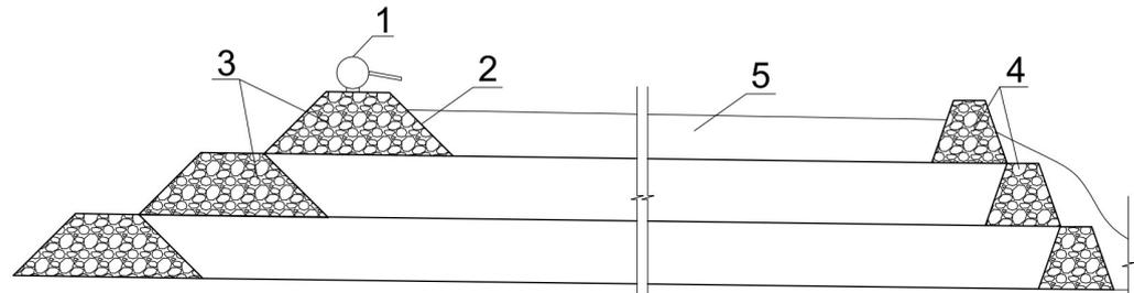
**Figure 4.** The scheme of the dam inwash: 1—distributive slurry pipeline; 2—geotextile anti-filtration screen; 3—a retaining slag prism of a dam; 4—slurry collecting slag prism; 5—inwashed tails.
