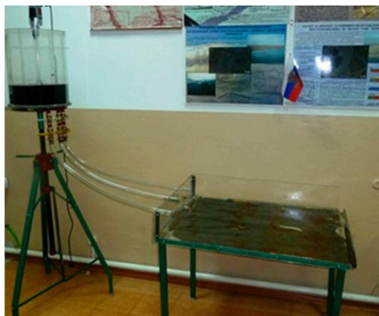
**Figure 9.** The design of a laboratory setup for modeling the alluvium of the tailing dam.
