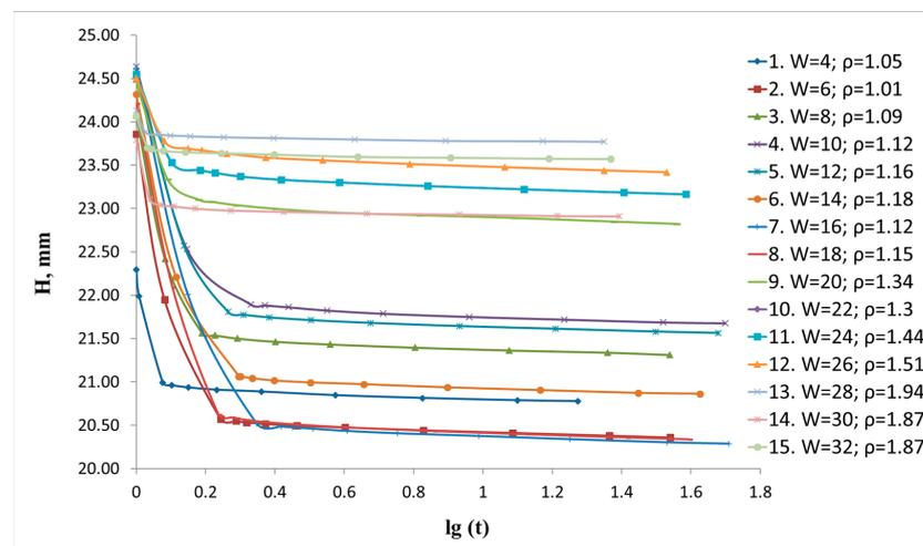
**Figure 19.** Compression curves for the tails samples with specified moisture content and density.
