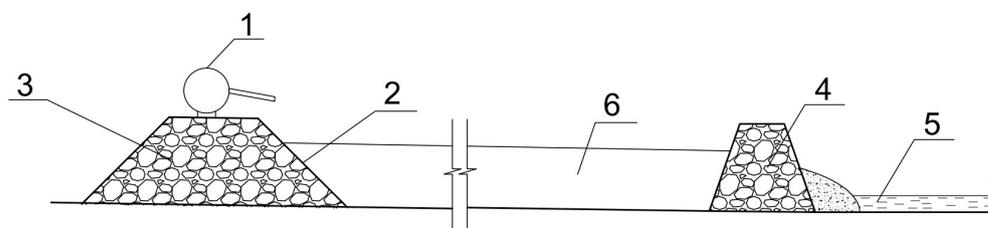
**Figure 3.** The scheme of the dam inwash: 1—distributive slurry pipeline; 2—geotextile anti-filtration screen; 3—the retaining slag prism of a dam; 4—slurry collecting slag prism; 5—pool; 6—inwashed tails.
