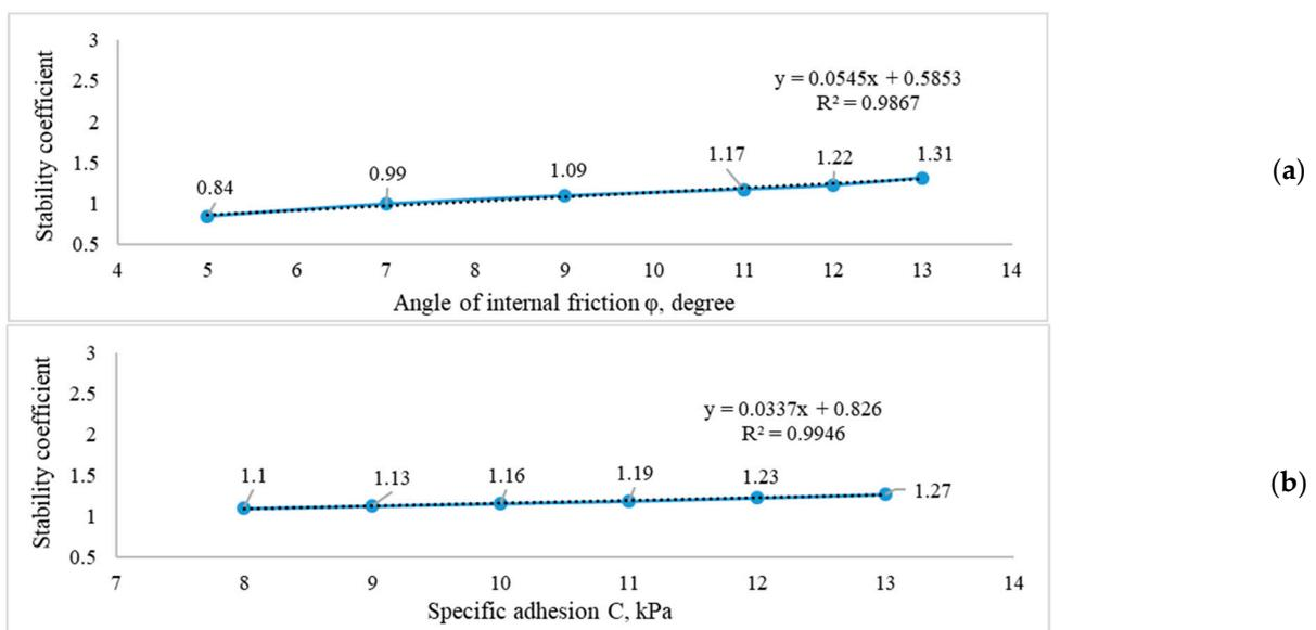
Figure 14. Influence of tailings strength characteristics on the dam’s stability coefficient: (a) angle of internal friction; (b) specific adhesion.
