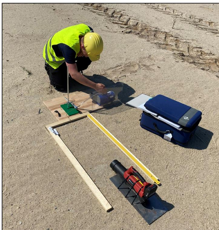
**Figure 5.** Test setup for dust emission measurements.
