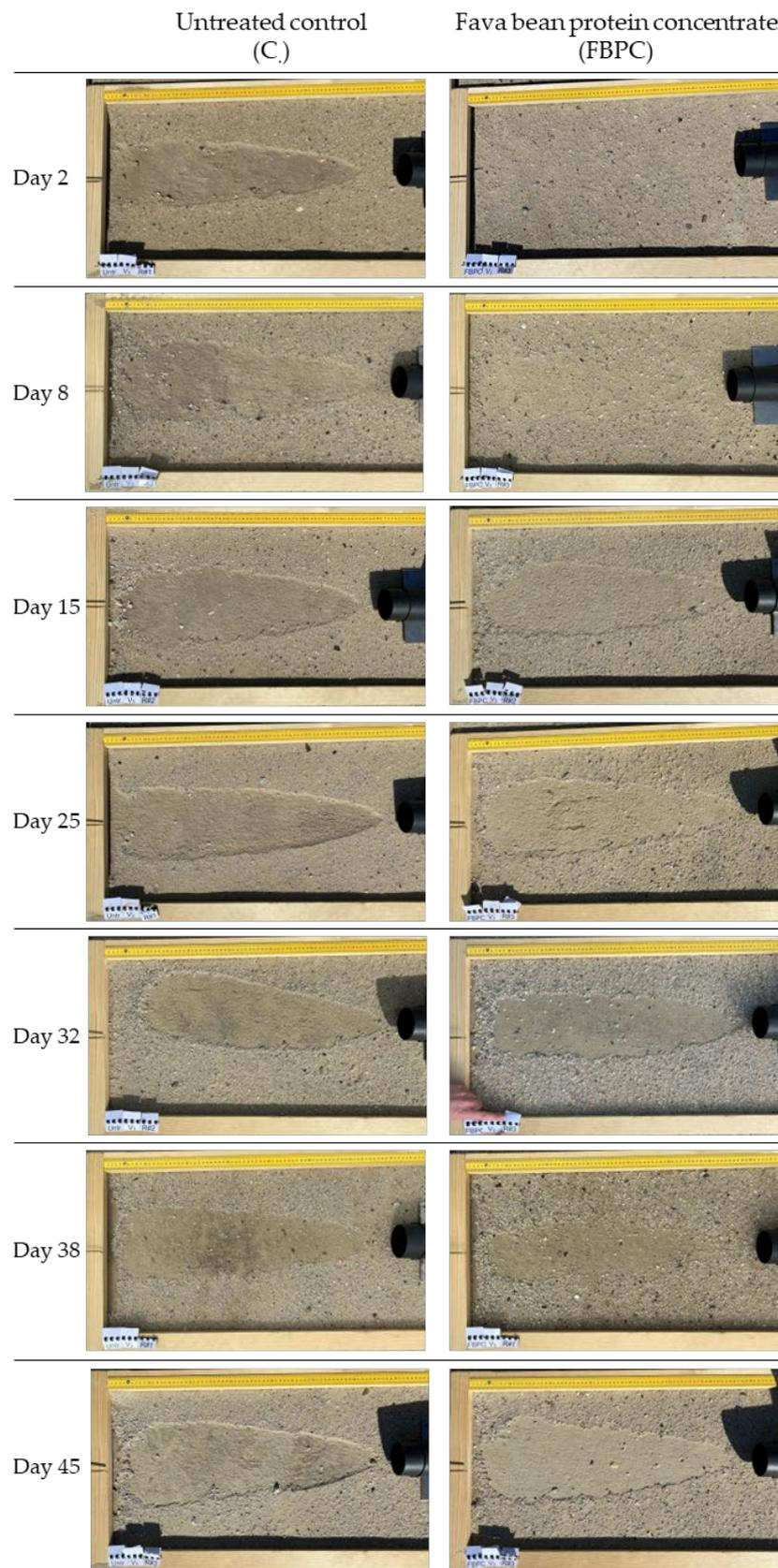
**Figure A3.** Exemplary photographs of untreated control (C) and FBPC-treated trial plots after subjecting them to air speed of  $v_3$  (17.4 m/s) for 60 s. The trial plots had dimensions of  $40 \times 70 \text{ cm}^2$ .
