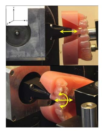
**Figure 1.** Resin model with aligner fitted in the orthodontic measurement and simulation system (OMSS): The tooth to be moved (Tooth 25) was adjusted in the aligned position in the aligner. Simulation of three tooth movements: intrusion/extrusion by 0.2 mm (X axes) (upper), oro-vestibular translation by 0.2 mm (Z axes), and  $2^{\circ}$  rotation around the tooth axis in disto-mesial direction (around X axes) (lower).
