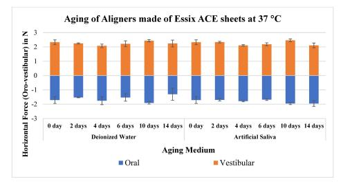
**Figure 3.** Mean of maximum oro-vestibular forces on tooth 25 generated by aligners made from Essix ACE<sup>®</sup> sheets after aging in deionized water and in artificial saliva at 37 °C.
