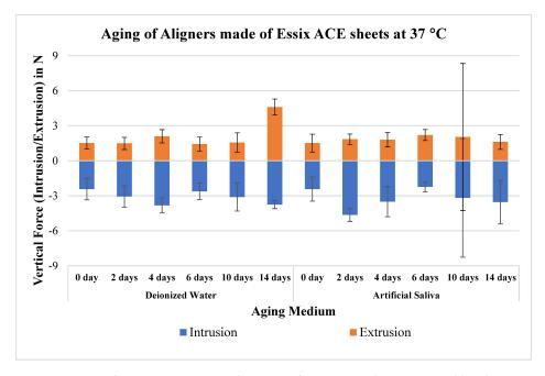
**Figure 2.** Mean of maximum intrusive/extrusive forces on tooth 25 generated by aligners made from Essix ACE<sup>®</sup> sheets after aging in deionized water and in artificial saliva at 37 °C.
