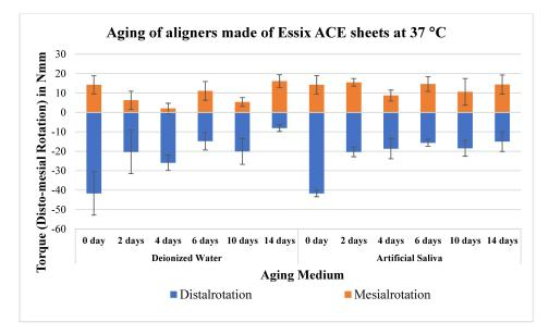
**Figure 4.** Mean of maximum torque upon rotation (disto-mesial rotation) around tooth 25 axes generated by aligners made from Essix  $ACE^{(B)}$  sheets after aging in deionized water and in artificial saliva at 37 °C.
