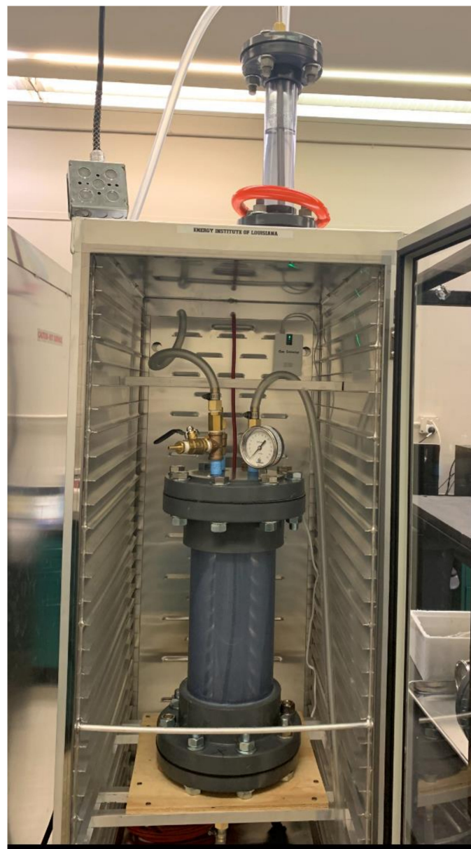
Figure 1. Laboratory-scale (8 L) digester unit for anaerobic digestion of synthetic wastewater.
