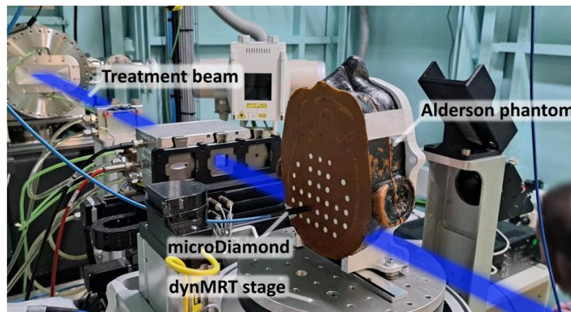
**Figure 4.** Alderson Radiation Therapy Phantom mounted on the dynamic MRT stage in Hutch 2B in the IMBL. The PTW microDiamond detector may be interchanged with any of the tissue-equivalent white plugs in the phantom. The blue region indicates the path of the incident radiation treatment beam.
