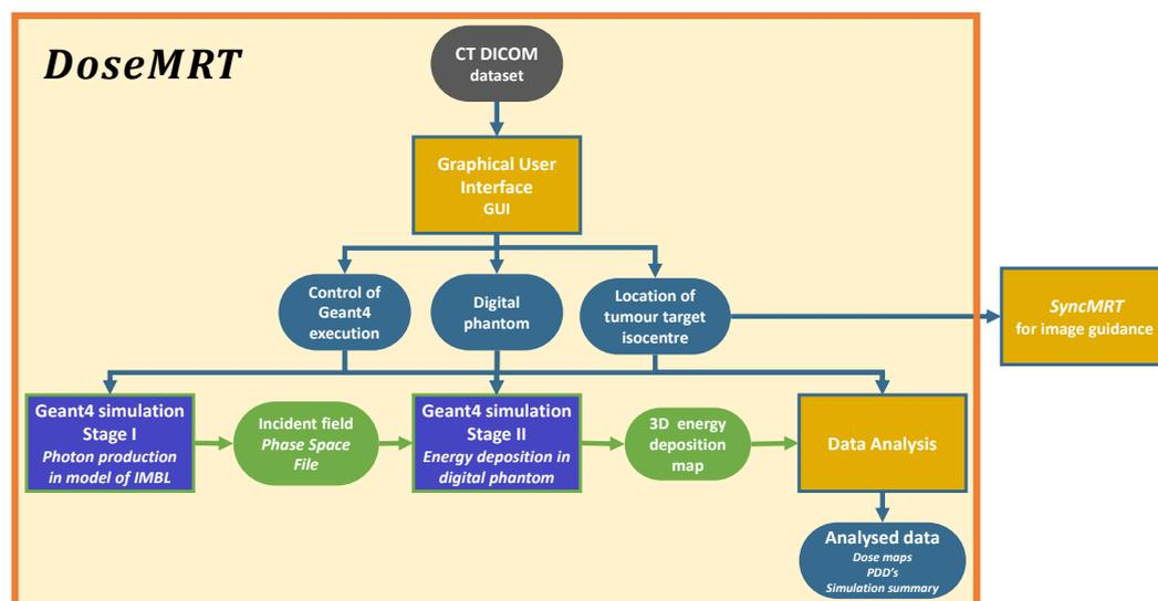
**Figure 1.** The *DoseMRT* simulation workflow. The user only needs to choose the treatment modality (broadbeam or MRT delivery, magnetic field intensity and filtering), input the patient digital phantom and the location of the tumour target isocentre through the Python GUI. The output of *DoseMRT* is 3D dose maps in the tumour target. Software calculation stages are indicated by square boxes, whilst the data passed between each stage are indicated with rounded borders.
