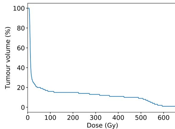
**Figure 9.** Cumulative distribution function of dose per unit volume over the entire planning target volume (tumour plus treatment margin), scaled to provide a minimum 10 Gy in the valley regions. The non-uniformity of dose distribution is characteristic of microbeam irradiation. The results were obtained with an MRT configuration of 50  $\mu\text{m}$  microbeams spaced with 400  $\mu\text{m}$  centre-to-centre.
