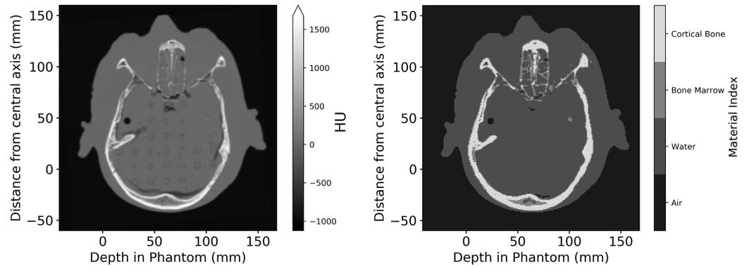
**Figure 2.** Axial slice of the Alderson Phantom, comparing the imported CT DICOM dataset (left) and the digital phantom produced after segmentation (right). Dimensions are given relative to the centre of the incident treatment beam and the surface of the phantom.
