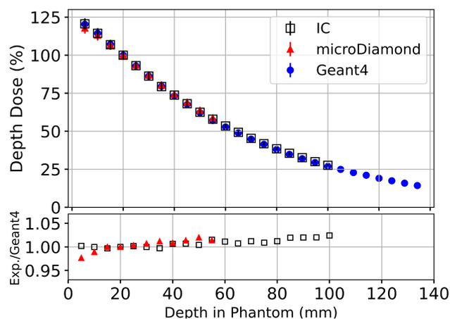
**Figure 5.** Percentage depth dose (PDD) measurements along the central axis of  $20 \times 20 \text{ mm}^2$  field performed in a  $14 \times 17 \times 12 \text{ cm}^3$  liquid water tank with PTW PinPoint 3D IC (Black), PTW microDiamond (Red) detectors and Geant4 simulations (Blue) normalised at a depth of 20 mm. The lower plot shows the ratio between the Geant4 simulation and experimental measurements using the PTW microDiamond and PTW Pinpoint 3D detectors.
