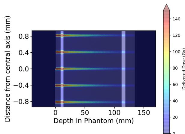
**Figure 7.** Geant4-simulated 2D dose map for five microbeams at the centre of the MRT treatment field in the Alderson Radiation Therapy Phantom. Microbeam simulations were performed using the entire phantom depicted in Figure 6; however, only the central five microbeams are displayed here for visual clarity.
