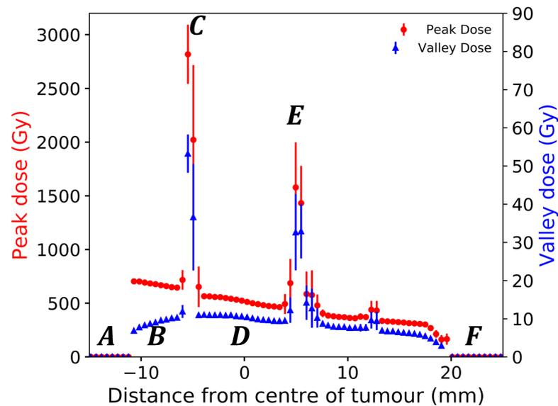
**Figure 11.** Geant4 simulated depth dose profiles for eight microbeam peaks and nine valleys at the centre of the treatment field in voxelised rat volume. The incident beam travels in the positive direction on the x-axis and traverses (A) air, (B) bolus and skin, (C) entry side skull, (D) brain and tumour, (E) exit side skull, soft tissue, and finally (F) air.
