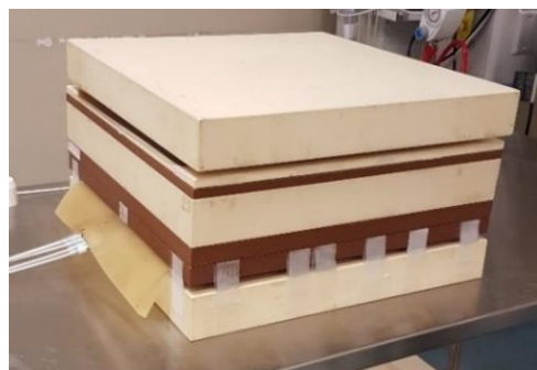
Figure 4. Dose rate dependence phantom. The phantom used to test OSLD dependence on dose rate. An additional 8 cm of solid water was added to the middle of the phantom to provide a total source-to-OSLD distance of 12 cm, as shown in this image.
