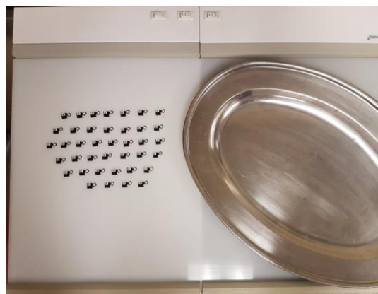
Figure 6. X-ray lightbox. Optical annealing set up with an array of 40 open OSLDs arranged on the surface of an X-ray lightbox.
