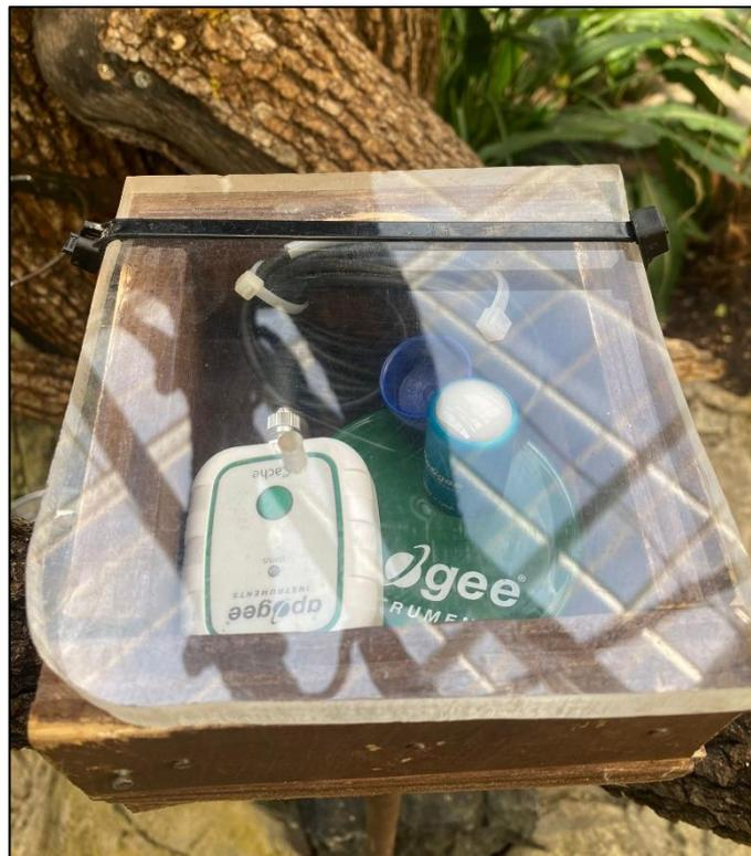
**Figure 3.** Detail of the light sensor placed inside the wooden tailor-made protective cage and the methacrylate protective cover. Biodomo—Parque de las Ciencias de Granada.
