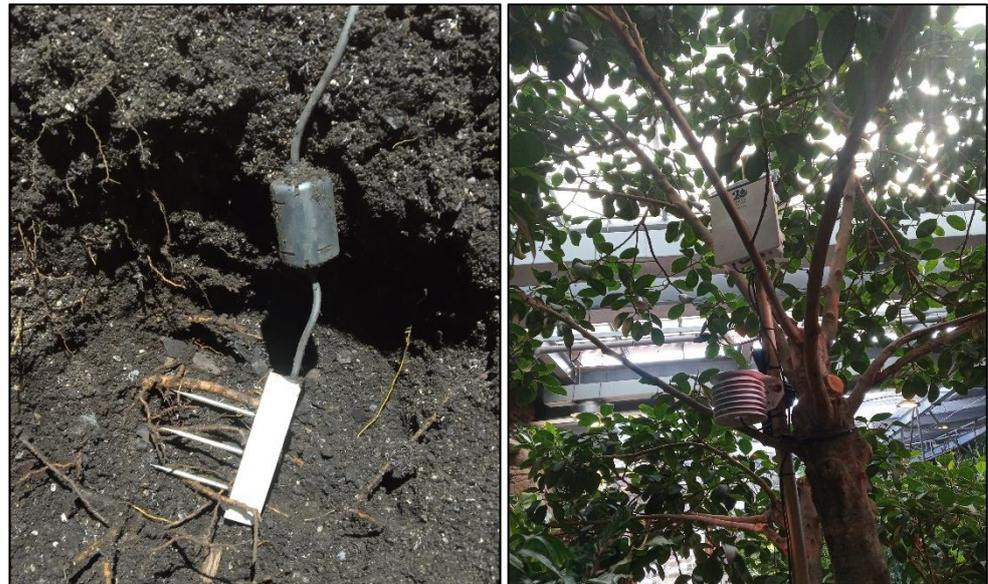
**Figure 4.** Detail of the ATMOS14 (left) and TEROS12 (right) probes. Biodomo—Parque de las Ciencias de Granada.
