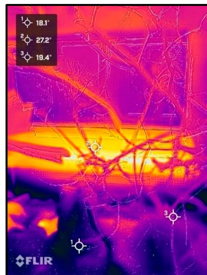
Figure 4. Image from the inside area of the C. obscurus enclosure. FLIR thermal image of bar heater reading 27.2 °C (as indicated by the white crosshairs numbered 2) and floor temperature reading 18.1–19.4 °C (as indicated by the white crosshairs numbered 1 and 3).
