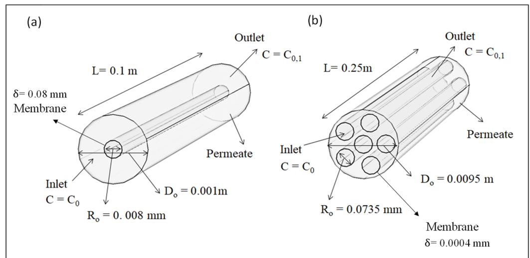
**Figure 3.** Schematic diagram of the single tube and HFM module. (a) Single hollow fiber case study for CO<sub>2</sub>/CH<sub>4</sub> separation (b) Multiple hollow fiber membrane module for N<sub>2</sub>/O<sub>2</sub> separation.
