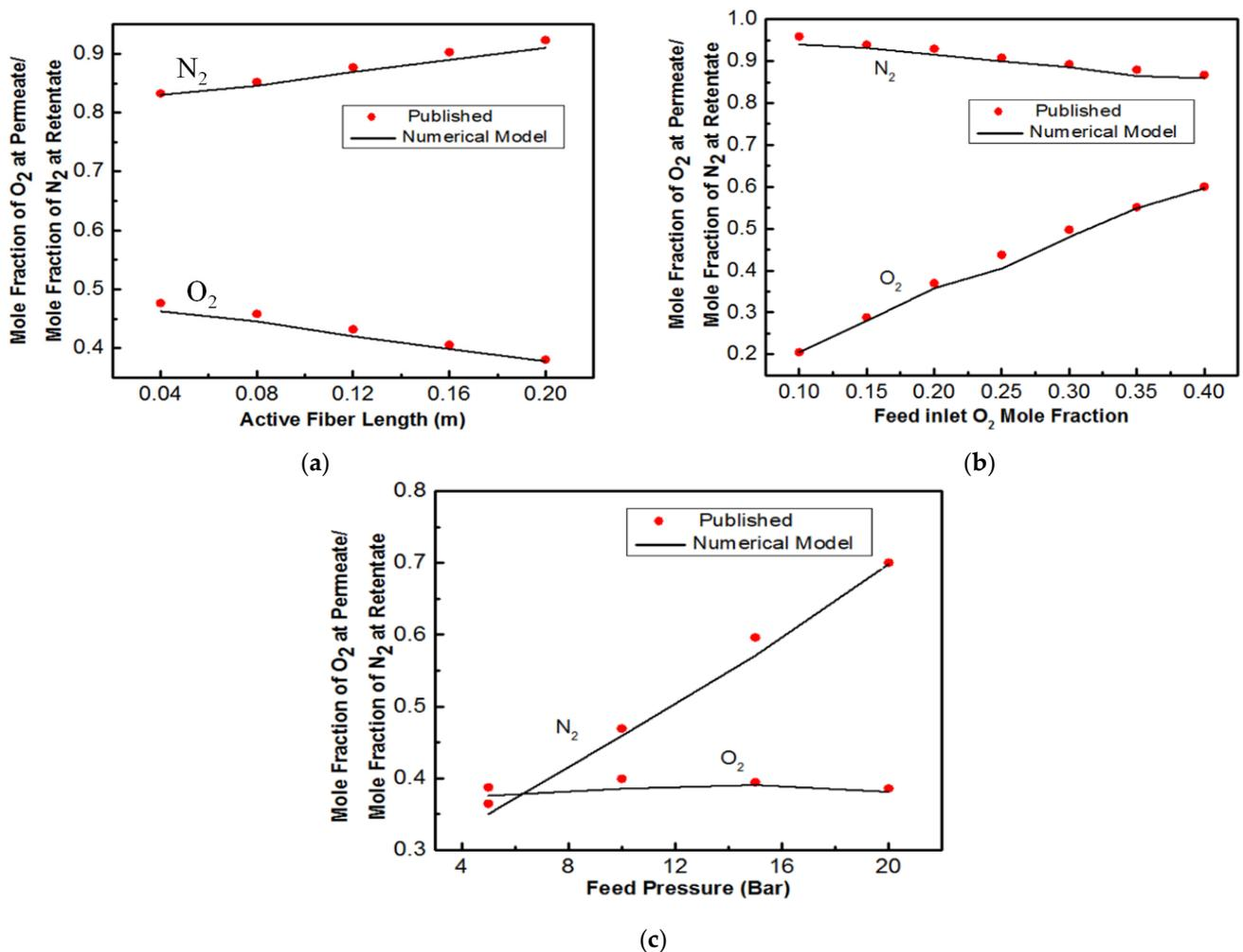
**Figure 7.** (a)  $O_2$  and  $N_2$  mole fraction variations with fiber length in HFM module; (b) mole fraction of  $O_2/N_2$  with fiber length in permeate and reject sides in HFM module (Reprinted with permission from Ref. [36]. 2016, Seyed Saeid) [36]; (c) feed mole fraction of the  $O_2/N_2$  in permeate and reject sides in HFM module (Reprinted with permission from Ref. [36]. 2016, Seyed Saeid) [36].
