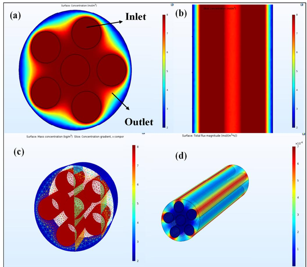
**Figure 5.** (a) Oxygen gas concentration in inlet and outlet side in HFM module; (b) 2-dimensional inlet oxygen concentration variation in the HFM module; (c) oxygen inlet variation as gradient high to low in the HFM module; (d) oxygen flux magnitude in HFM module.
