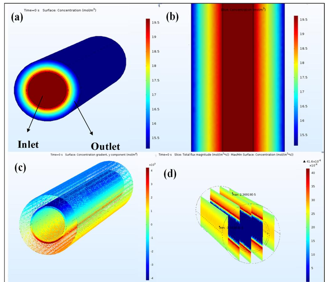
**Figure 6.** (a) Inlet gas  $CO_2$  concentration in inlet and outlet sides in HFM module; (b)  $CO_2$  2-dimensional gas variation model in HFM module; (c)  $CO_2$  gas inlet variation as gradient high to low in HFM module; (d)  $CO_2$  flux magnitude in HFM module.
