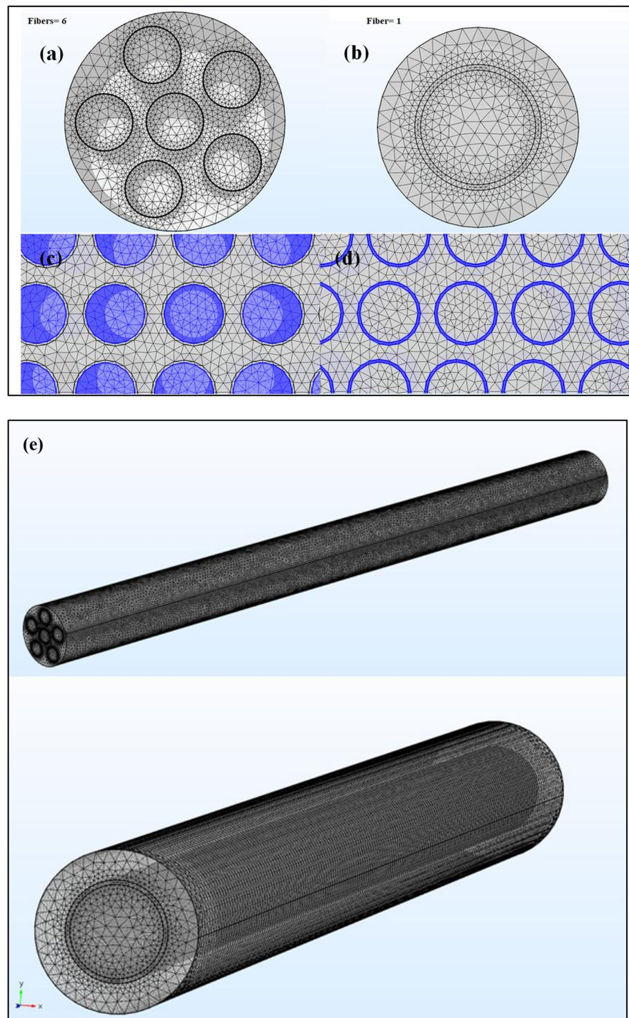
**Figure 4.** (a) Meshing of HFM membrane module for six fibers; (b) the meshing of single-tube HFM module; (c) fiber-lumen side meshing for inlet flow in the HFM module; (d) membrane thickness meshing; and (e) 3-D meshing of both single and six fiber HFM.
