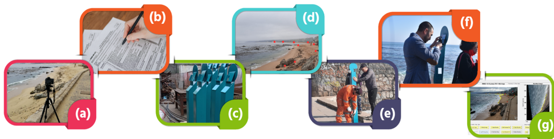
Figure 2. Workflow CoastSnap implementation in Valparaíso region, Chile. (a) Selection of the installation sites; (b) request for permits from the councils to install the platforms; (c) design, signaling, and construction of the platforms; (d) control points with GPS; (e) installation of the platforms; (f) inauguration and start-up; and (g) extraction and processing of shoreline, from open-source code. Source (b image creative commons from canvas for educational).
