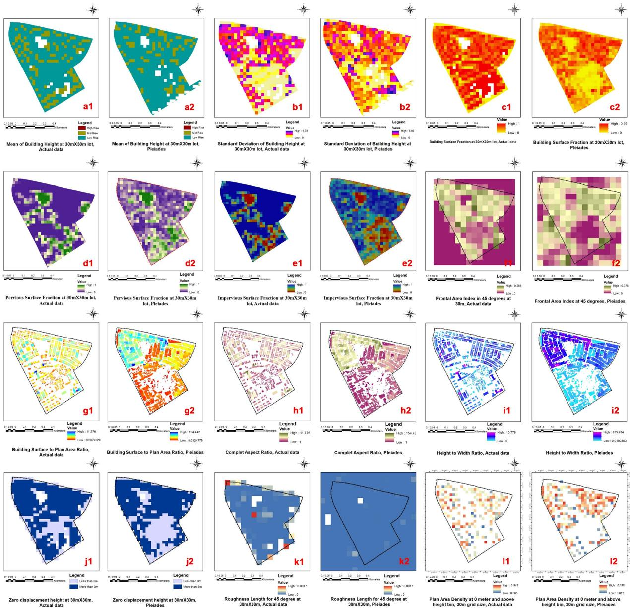
**Figure 5.** UCPs derived using satellite data (1) and reference data (2): (a) MBH; (b) SDBH; (c) BSF; (d) PSF; (e) ISF; (f) FAI;(g) BSPAR;(h) CAR;(i) H/W Ratio; (j)  $Z_d$ ; (k) RL;(l) PAD.
