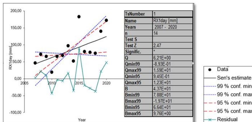
**Figure 2.** Example of the application of the Sen’s slope ( $f = Qt + B$ ) and Mann-Kendall method to the yearly time series of the RX1day index for the Souda meteorological station. A positive (negative) Z number indicates a positive (negative) trend. By Q and B, the slope of the trend and intercept are denoted along with the 95% and 99% confidence levels, respectively. In case the trend is statistically significant, it is marked with a star (\*).
