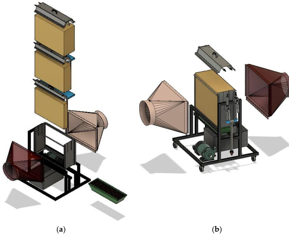
**Figure 1.** Exploded view of the test bench (a) with the three possible pad thickness and (b) a 300 mm thick pad.
