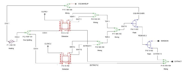
Figure 1. Simulation diagram developed in the SuperPro Designer 10 simulation interface.
