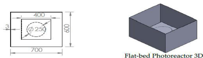
Figure 2. Different views of the dimensions of the photoreactor.
