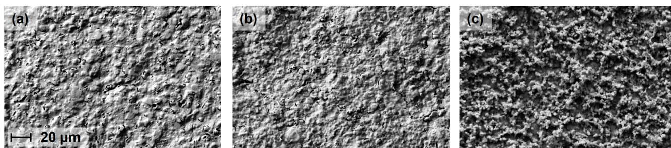
Figure 1. SEM pictures of (a) blank electrode, (b) polythiophene thin film that was electropolymerized under the optimized conditions described in the method section, (c) rough polythiophene film electropolymerized by a 6\times higher current density. Scale bare is applicable to all pictures.
