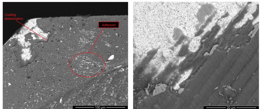
**Figure 1.** TiAlN-coated tool after 2 m cutting length and 480 mm/min feed rate (on the left) and TiAlSiN-coated tool after 4 m cutting length and 480 mm/min feed rate (on the left).
