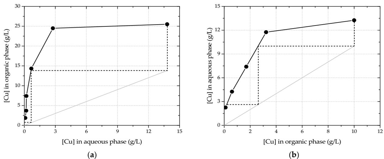
**Figure 2.** (a) McCabe–Thiele extraction diagram at equilibrium pH 1.5. The A/O ratio for the operation line is 1:1. (b) McCabe–Thiele stripping diagram with 2 M HCl. The A/O ratio for the operation line is 1:1.
