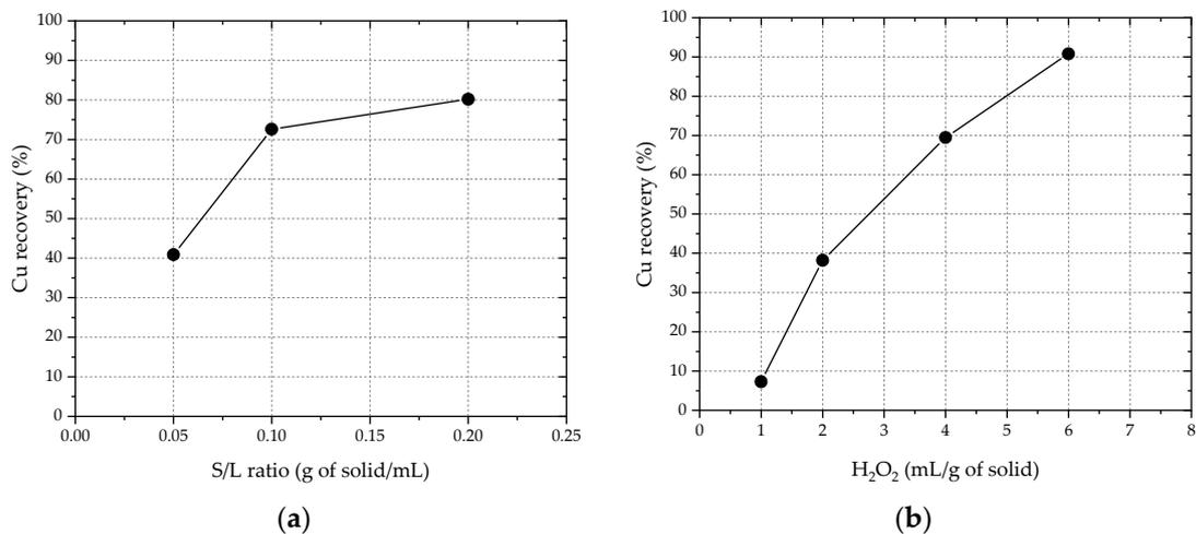
**Figure 1.** (a) Effect of the S/L ratio on Cu recovery, using 2 M H<sub>2</sub>SO<sub>4</sub> and 1 mL H<sub>2</sub>O<sub>2</sub> (30% w/w)/g of copper dust. (b) Effect of the H<sub>2</sub>O<sub>2</sub> concentration (mL of oxidant/g of dust) on Cu recovery, using 2 M H<sub>2</sub>SO<sub>4</sub> and an S/L ratio of 0.1 g/mL.
