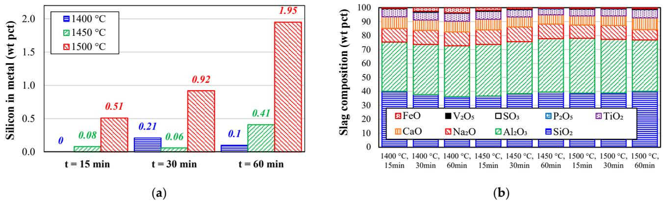
**Figure 4.** The effects of temperature and time at 7% carbon addition on (a) silicon in metal; and (b) slag composition.
