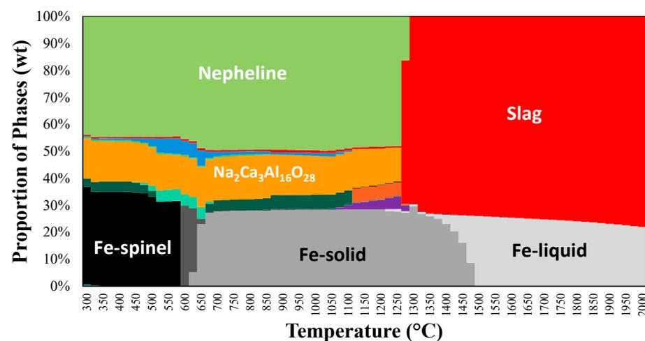
**Figure 2.** Type and proportion of phases as a function of temperature from reduction at 7% carbon + 5% LLDPE addition based on FactSage calculation.
