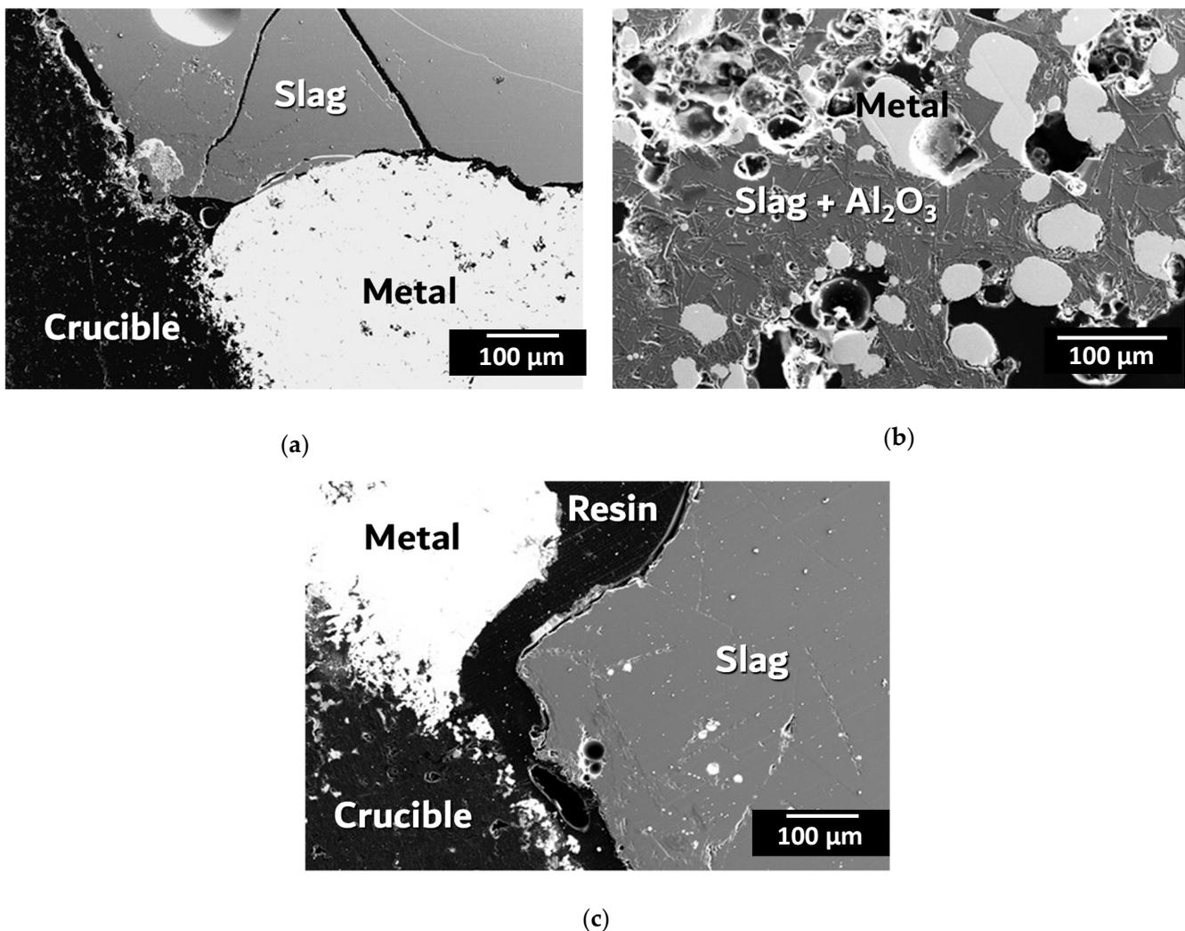
**Figure 3.** Microstructures of quenched samples from experiments at  $T = 1450\text{ }^{\circ}\text{C}$  and  $t = 60$  min with: (a) 7% carbon addition; (b) 14% carbon addition; and (c) 7% carbon + 5% LLDPE addition.
