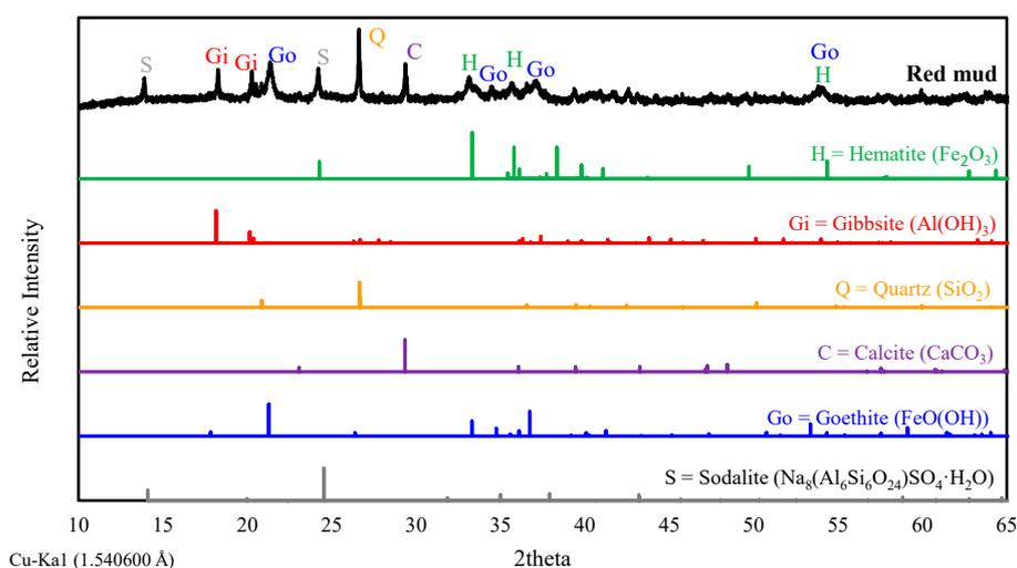
**Figure 1.** X-ray diffraction pattern of red mud.
