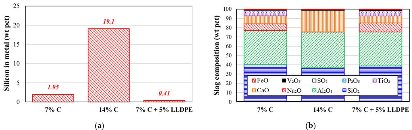
**Figure 5.** The effects of carbon and LLDPE additions at  $T = 1450\text{ }^{\circ}\text{C}$  and  $t = 60\text{ min}$  on: (a) Silicon in metal; and (b) Composition of slag.
