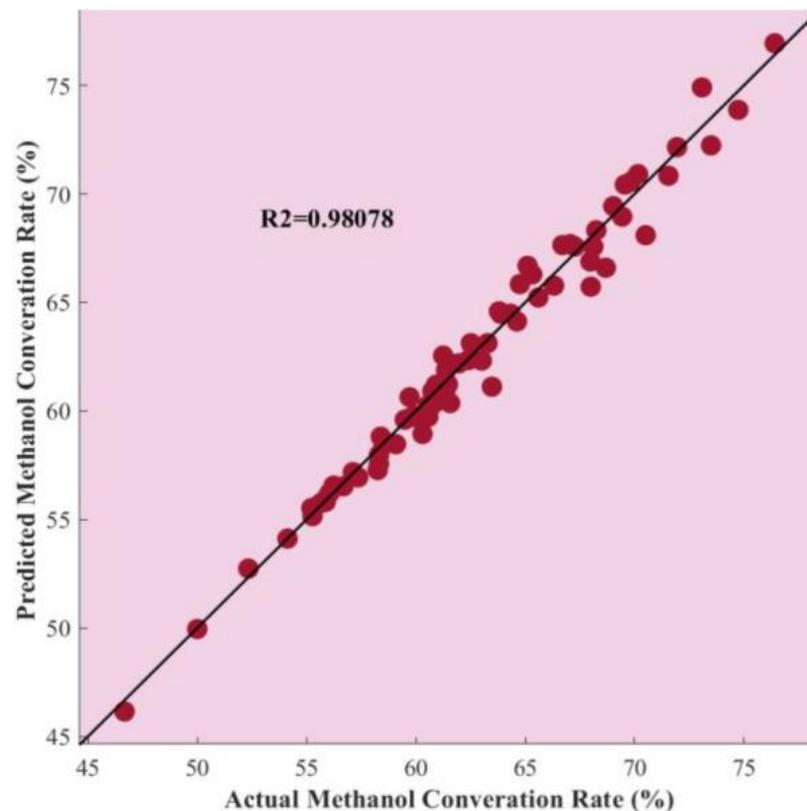
**Figure 1.** Actual vs. predicted methanol conversion rate.
