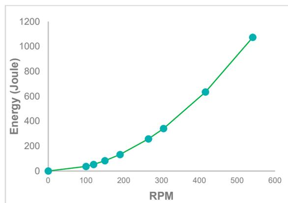
**Figure 5.** Relationship between RPM and energy stored in flywheel.
