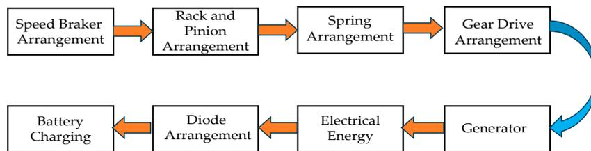
Figure 3. Block diagram of electrical energy generation.
