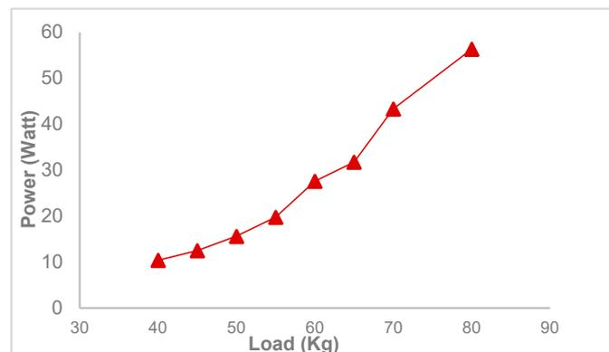
**Figure 4.** Relationship between applied load and power generated from the system.
