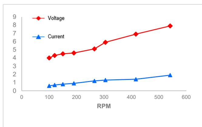
**Figure 6.** Relationship between voltage and current generated with respect to RPM.
