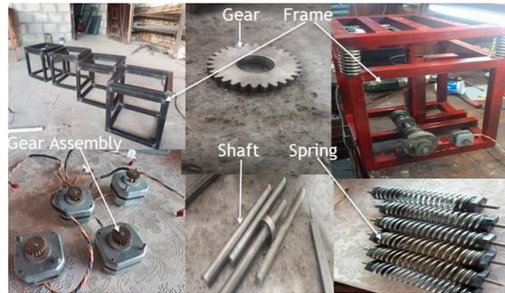
Figure 1. Different components of power generation system.
