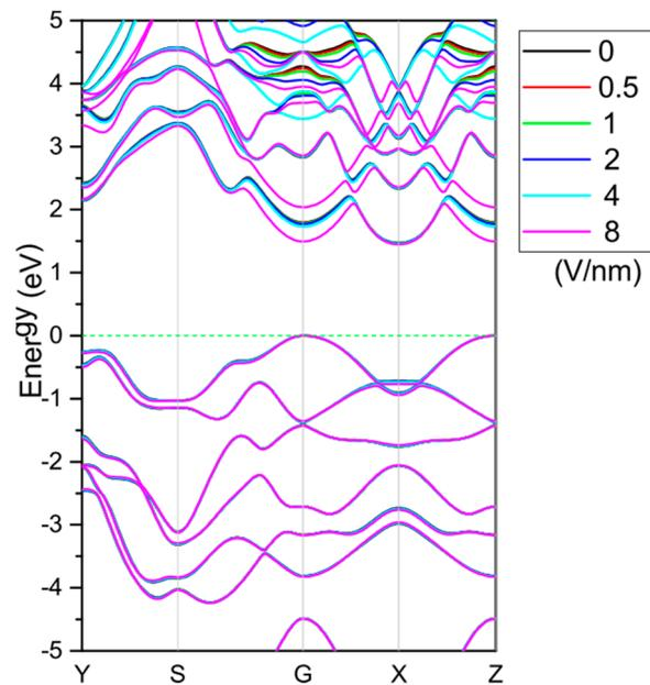
**Figure 4.** The effect of an electric field on the band structure of monolayer GeSnS<sub>2</sub>.
