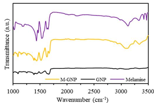
**Figure 2.** FTIR spectra of melamine, GNP, and M-GNP.
