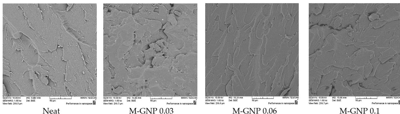
Figure 6. SEM micrographs of the tensile fracture surface.
