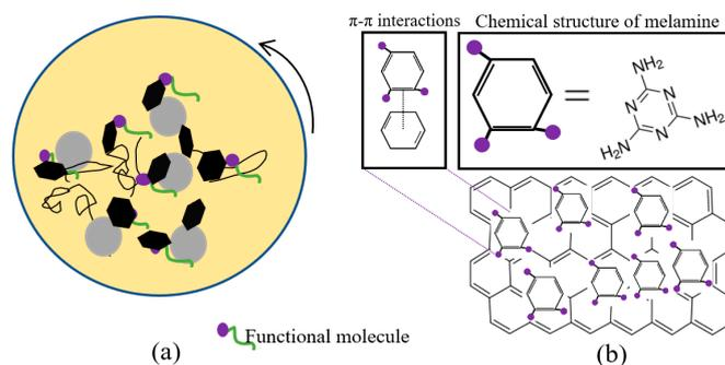
**Figure 1.** Functionalisation process of GNPs: (a) Schematic illustration of shaking and ball-milling process and functional molecules. (b) Schematic illustration of the functionalisation of GNP with melamine.
