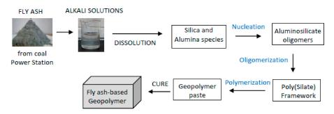
Figure 1. The transformation process of fly ash into a binder for geopolymer materials [10,11].
