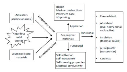
Figure 2. Geopolymerization process and geopolymers applications [16].
