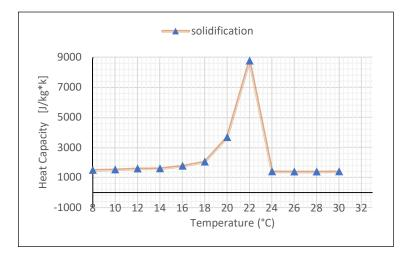
Figure 3. Mass thermal capacity of Micronal<sup>®</sup> PCM SmartBoard<sup>TM</sup> 23, cooling stage: 30–8 °C.
