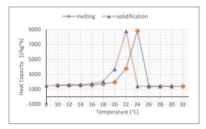
Figure 4. Thermal capacity of Micronal<sup>®</sup> PCM SmartBoard<sup>TM</sup> 23 for melting and cooling stages.
