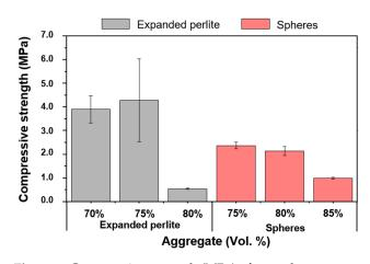
**Figure 4.** Compressive strength (MPa) of geopolymer composites varying the amount of expanded perlite and geopolymer spheres.
