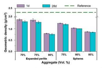
**Figure 3.** Geometric density of geopolymer composites varying the amount of expanded perlite and geopolymer spheres (measured on the 1st and 28th day). Reference means the control specimen without addition of lightweight aggregate.
