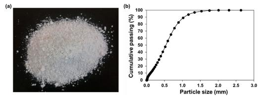
Figure 1. (a) Expanded perlite aggregate and its (b) particle size distribution.
