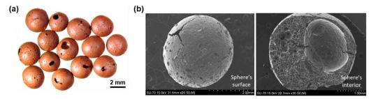
Figure 2. (a) Optical microscopy and (b) SEM micrographs of the red mud-based geopolymer spheres.
