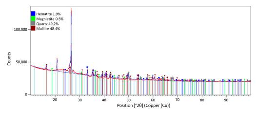
Figure 2. Diffractogram for fly ash.
