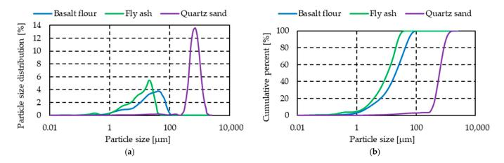
**Figure 3.** (a) The particle size distribution curves for fly ash, quartz sand, and basalt flour; (b) the cumulative curves for fly ash, quartz sand, and basalt flour.
