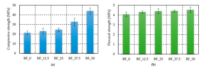
Figure 5. Results for tested geopolymers of (a) compressive strength test, (b) flexural strength.
