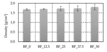
Figure 4. The density of the tested geopolymers.
