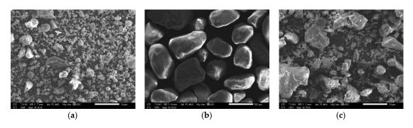
Figure 1. SEM micrographs of (a) fly ash, (b) quartz sand, (c) basalt flour.
