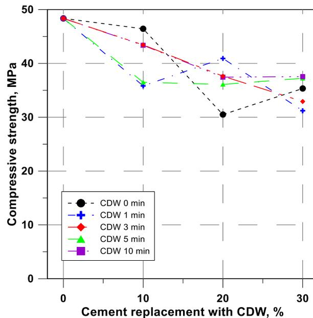
Figure 3. Results of compressive strength measurements.
