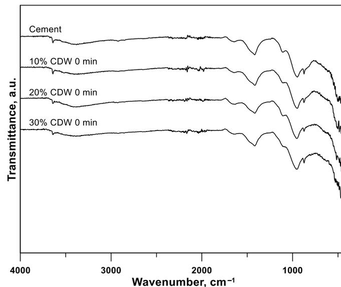
Figure 4. FTIR spectra of samples with different CDW content.
