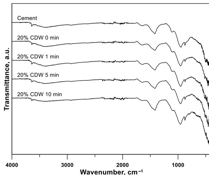
**Figure 5.** The FT-IR spectra of specimens (cement replacement with 20% CDW).
