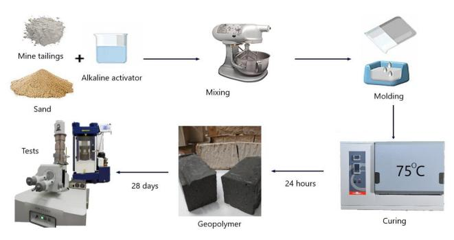
Figure 1. Scheme for sample preparation.
