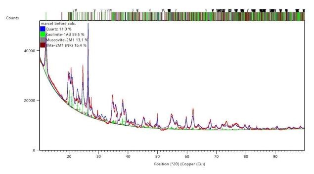
Figure 3. XRD analysis for coal shale from Marcel mining (before calcination).
