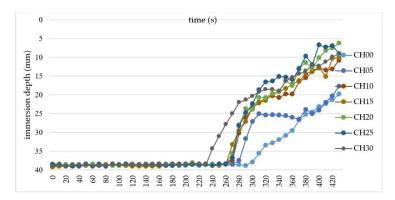
Figure 2. Cement-based mortar setting times.
