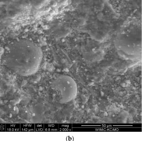
Figure 3. SEM micrographs of the 60PC-20GBFS-15SFA cement paste after (a) 2 days and (b) 28 days.
