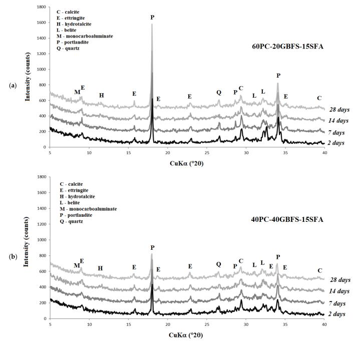
**Figure 2.** XRD patterns of the (**a**) 60PC-20GBFS-15SFA and (**b**) 40PC-40GBFS-15SFA cement pastes after 2, 7, 14, and 28 days.
